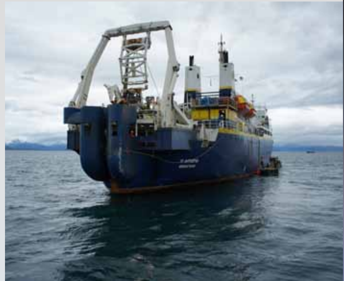
Over 80 miles of fiber-optic was laid in a trench at the bottom of an arctic inlet. The IT Intrepid was enlisted to trench the sea floor.
